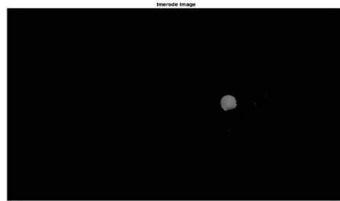
Fig. 12. Color-filtered image after passing through an erosion and a dilation filter
